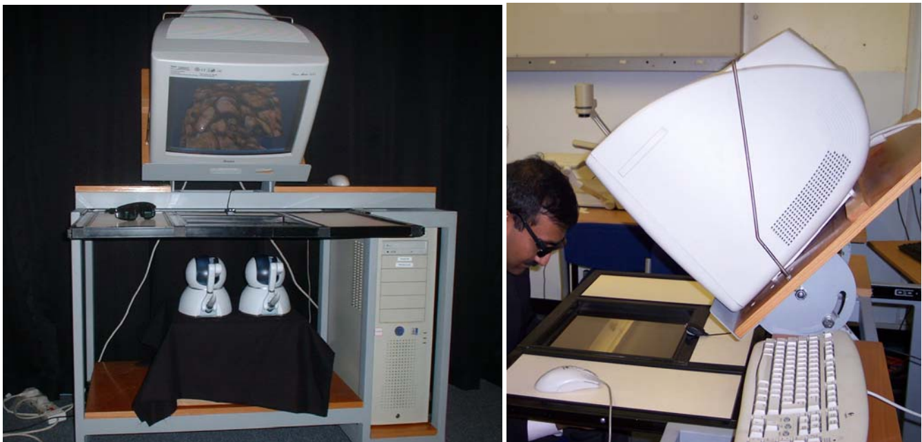
Figure 3: The physical design of our simulator (left) and typical operating position (right)
